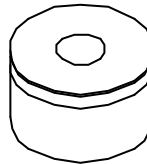
102247948601 REFLECTING BOARD (DIA. = ø5.5) PAN, MV2
